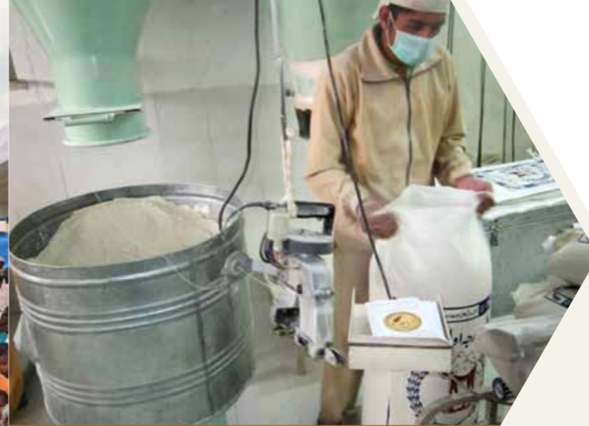
A worker adding iodine to salt in a factory, as part of a large-scale Food Fortification Programme in Afghanistan, funded by the Khalifa bin Zayed Al Nahyan Foundation and implemented by the Global Alliance for Improved Nutrition (GAIN). (Source: Khalifa bin Zayed Al Nahyan Foundation)
